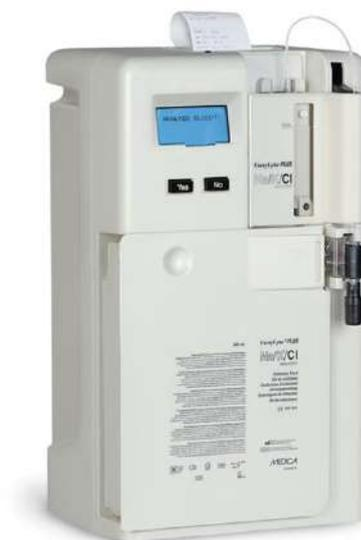
Gambar 2.1 Alat Easylyte Analyzer Metode ISE
